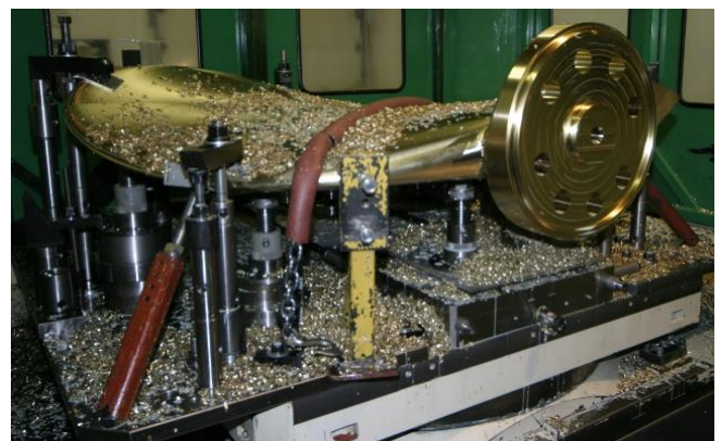
Fig. 5, Finish machining of the blade trunnion
