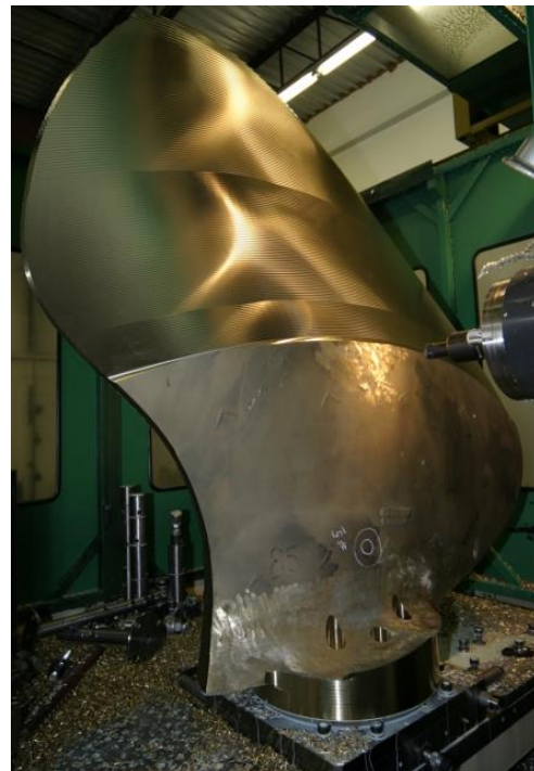
Fig. 3, Rough milling of the blade surfaces
