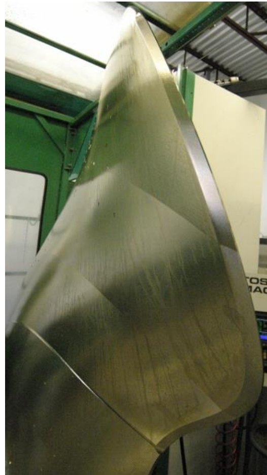
Fig. 9, Anti-singing chamfer finish machined with back surface. Bands 1, 2 and 3.
